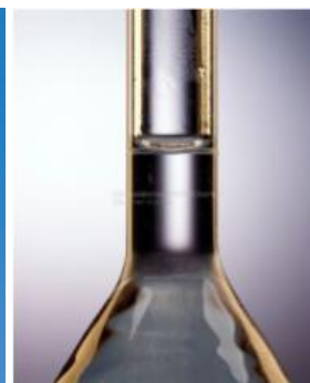
A volumetric flask filled exactly to the mark.
